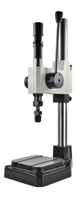
The manually operated spring impact press BM20 was designed for continuous industrial use and develops an adjustable impact force up to a maximum of  $3000 \, \text{kg}$  /  $30 \, \text{kN}$ . It is ideal for a whole range of applications such as stamping, embossing, riveting and caulking. The simple marking with one stroke enables a uniform marking depth even with parts of different heights.
