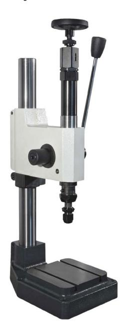
The manually operated spring impact press BM32 was designed for continuous industrial use and develops an adjustable impact force up to a maximum of  $6500 \, \text{kg}$  /  $65 \, \text{kN}$ . It is ideal for a whole range of applications such as stamping, embossing, riveting and caulking. The simple marking with one stroke enables a uniform marking depth even with parts of different heights.
