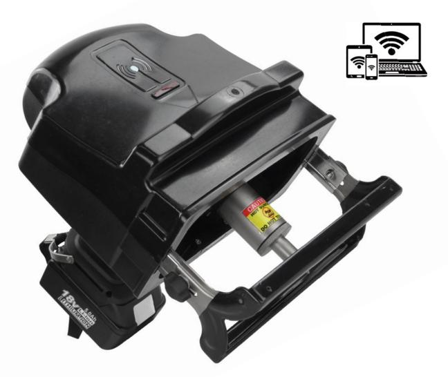
The battery operated BM155 Mobile Portable dot marking unit is characterized by its low weight, ease of use, good marking depth and high marking speed. The portable dot marking unit offer reliable and unchangeable markings directly into the material of the workpiece. The markings, which can consist of text, logos and data matrix codes, are created from of a series of needle points.
