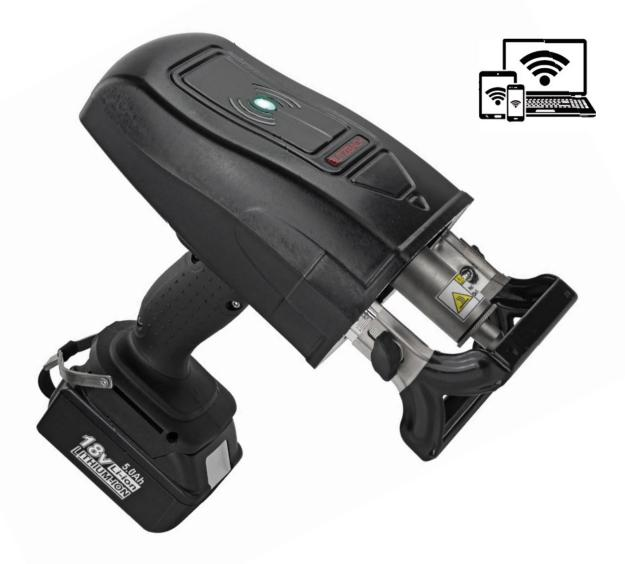
The battery operated BM53 Mobile Portable dot marking unit is characterized by its low weight, ease of use, good marking depth and high marking speed. The portable dot marking unit offer reliable and unchangeable markings directly into the material of the workpiece. The markings, which can consist of text, logos and data matrix codes, are created from of a series of needle points.
